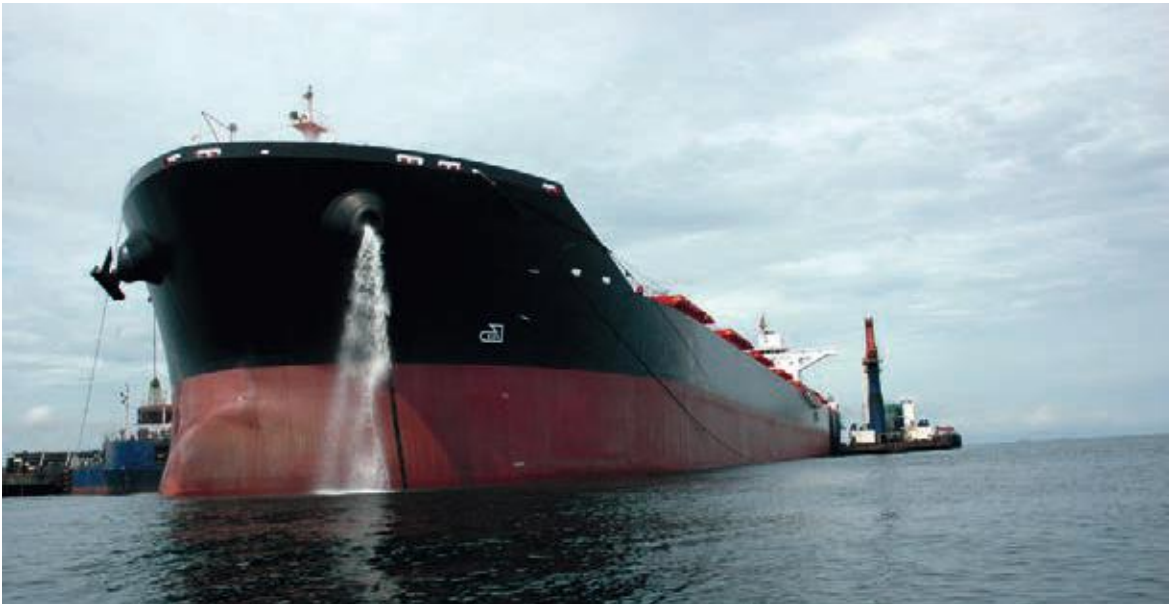
IMO's ballast water convention requires vessels to exchange ballast water at sea, which can result in high stress on the hull, especially if procedures are not correctly followed.
